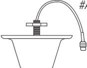
The Wideband Indoor Dome Server Antenna receives and transmits signal in a 360° pattern
